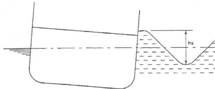
1. If  $h_s \geq 4.0$  metres, height of water on deck is calculated as per figure 3.
