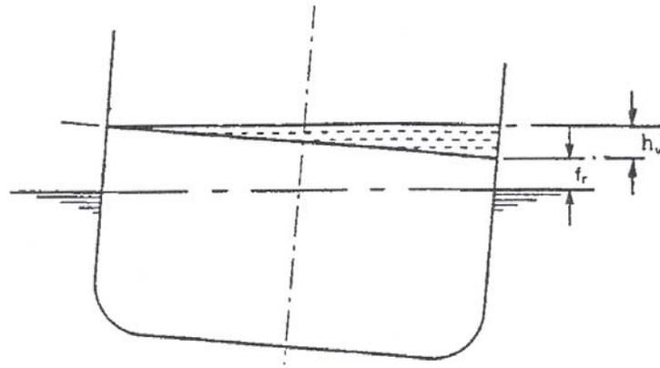
1. If  $f_r \geq 2.0$  metres, height of water on deck ( $h_w$ ) = 0.0 metres.
