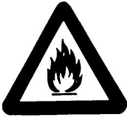
Flammable material or high temperature (1)
