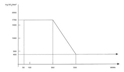
B.  $SO_2$  emission limit values expressed in mg/Nm<sup>3</sup> ( $O_2$  content 3%) to be applied by new plants with the exception of gas turbines:
